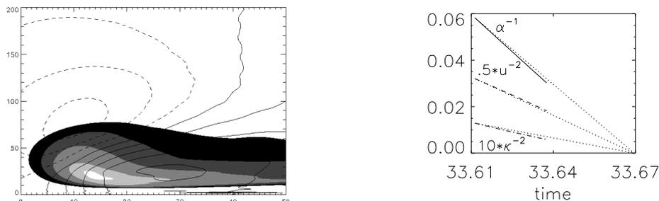
Figure 1: (Left): Plot of vorticity contours (gray scale) and stretching contours (lines) on the symmetry plane. (Right): Time dependence of quantities from vortex dipole approximation: maximum stretching (solid line), approaching velocity of vortices (dashed), and maximum curvature (dash-dotted). The dotted lines are just indicators.
