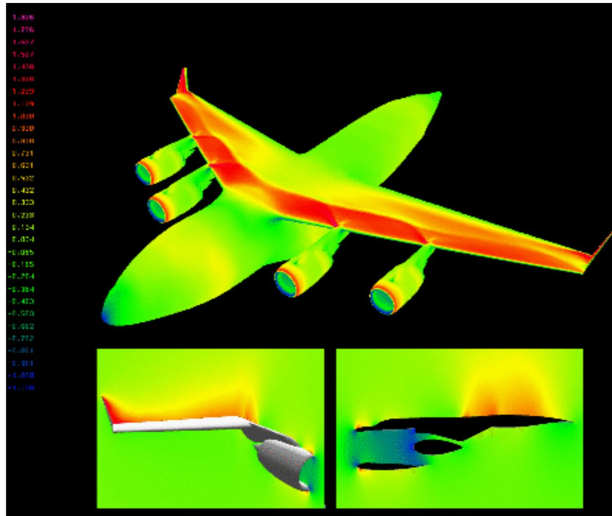
The Euler equations with the equations of energy and continuity are often solved by finite differences whereby the values of each velocity component, the density, and the internal energy are computed at each point. From these quantities constitutive relations (perfect gas law or isentropic pressure relation) are used to find pressure.
