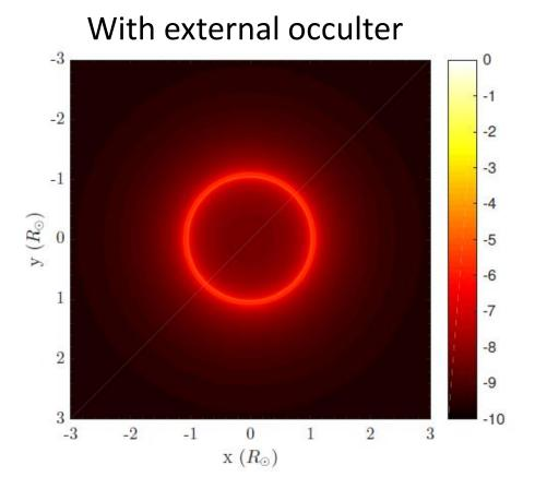
Intensity in plane D, final focal plane with the detector
