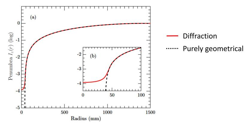
• The serrated (or saw-toothed ) occulter  $\Delta$ =20mm
