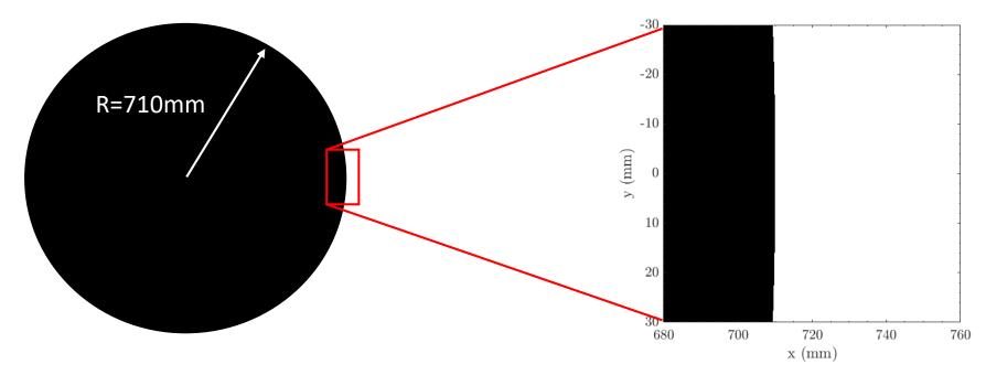
Occulting ratio of 1,05 solar radius at  $z_0$ =144m
