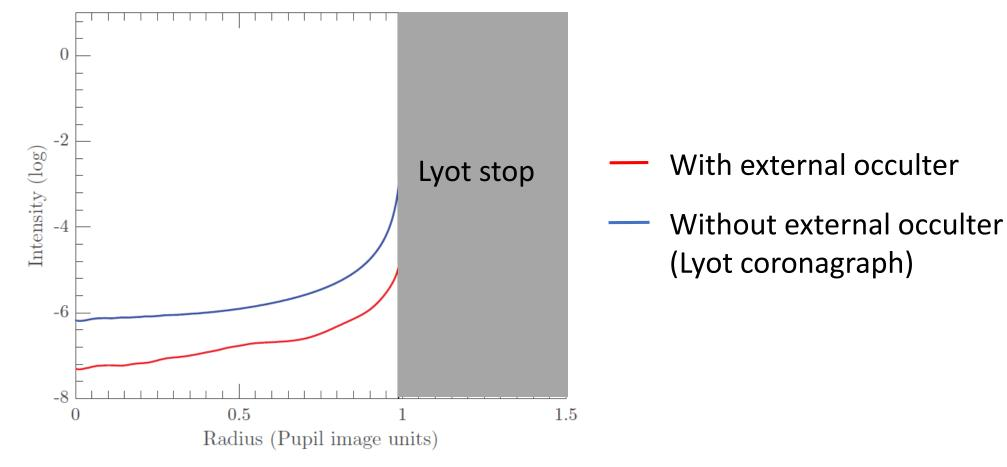
• Intensity in plane D, final focal plane with the detector
