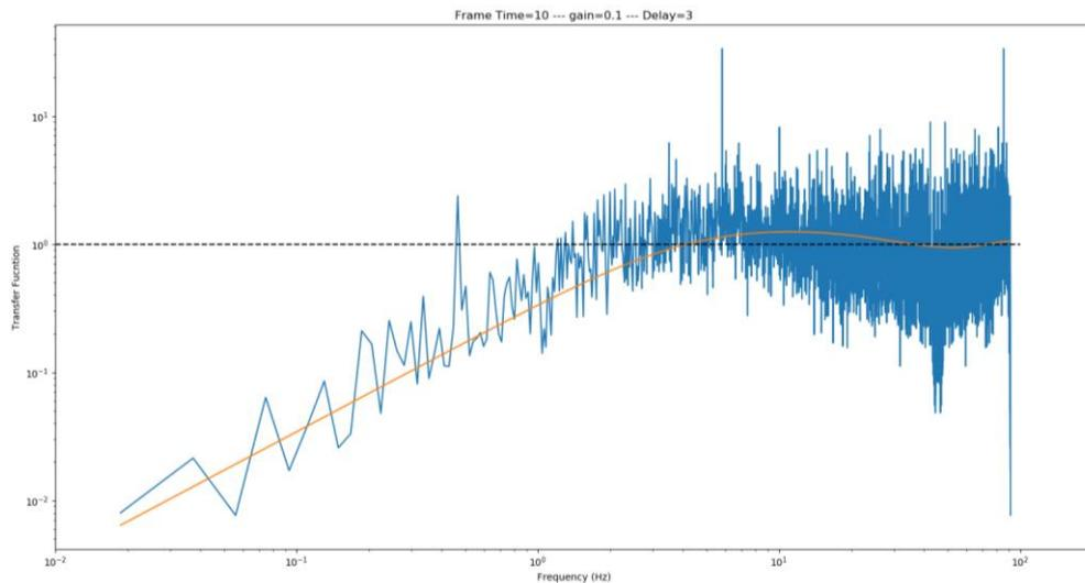
Figure 9: Transfer Function of the control loop with STS - Comparison with the transfer function of a pure integrator with a delay of 3 frames and a gain of 0.1
