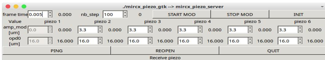
Figure 2: The `mircx_piezo_gtk` allows to start modulation on the PZT of the STS. The modulation are triangular. At the end of the modulation, the PZT return back to the reference position of  $16\mu\text{m}$ .
