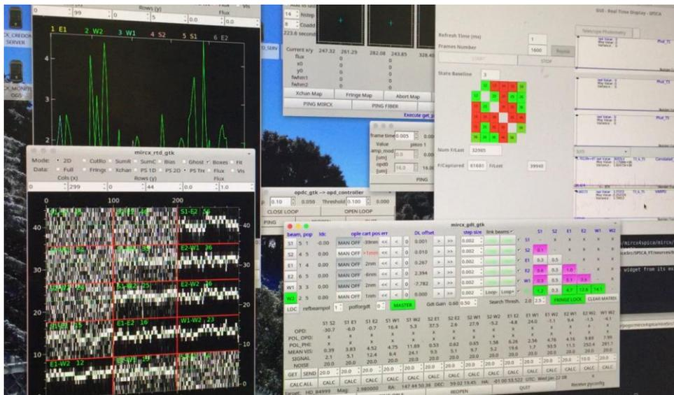
Figure 10: Left and bottom: MIRCx-RTD (15 waterfalls of Power Spectrum): 10 fringes are seen in this part of the figure. Bottom Right: the MIRCx GDT allowing to control the servo loop on the delay line: again 10 fringes are either green or pink (depending on instantaneous SNR). Upper-right: the RTD of the OPDC as developed for the integration and the tests and presenting detailed plots of the photometry, the variance of the phase, the group delay... and the status matrix.
