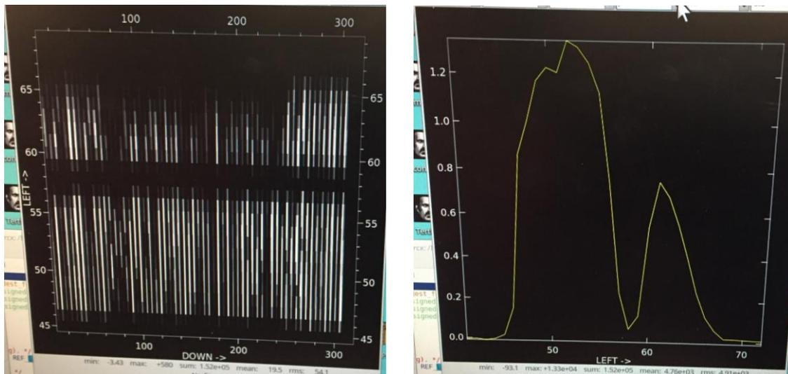
Figure 9: Raw image and spectrum with PRISM50. J band is on top (left figure) and on right (right figure)
