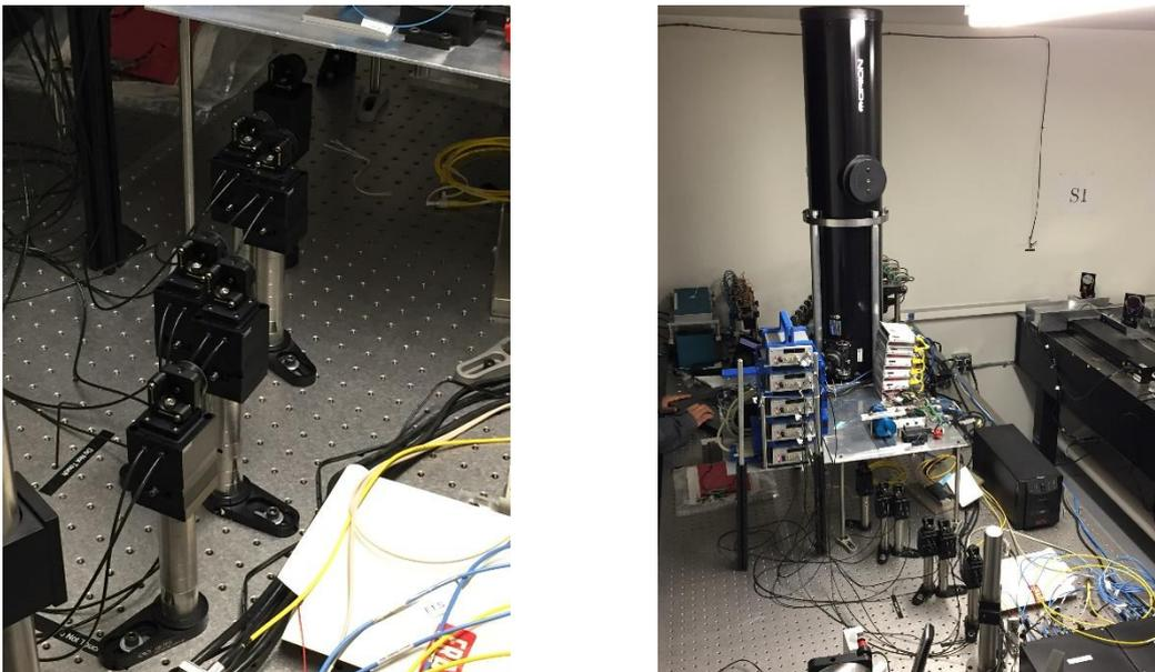
Figure 1: Left: The 6 new mounts supporting the OPD mirrors of the STS. Mirrors are the same as the previous ones. Right: General view of the STS, including the new electronics for the PZT (PZT controllers, DNA system). A new CHARA server (*mircx\_piezo\_server*) is in place and in charge of managing the communication with the hardware. Some commissioning GUIs have been used, their integrations into the STS GUI should be considered for the future use of these devices.
