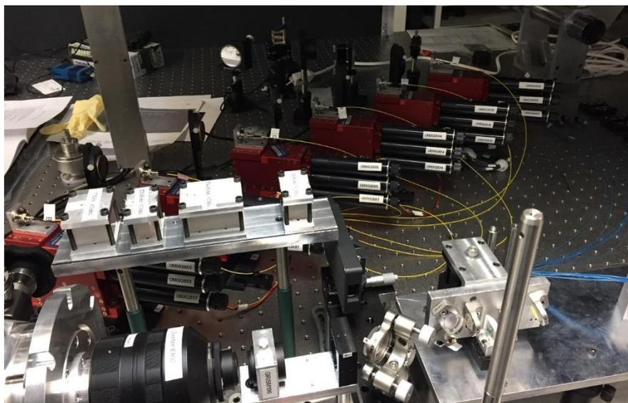
Figure 3: Installation of the SPICA-FT IO Chip in front of the MIRCx spectrograph. The 6 SPICA-FT fibers (yellow jacket) are connected to the MIRCx OAP injection modules. The IO Chip is installed inside a grey box supported by a goniometric mount. A tip/tilt flat mirror permits to align the outputs of the chip on the detector. The focus is made by manually moving the whole plate in the direction of the spectrograph.
