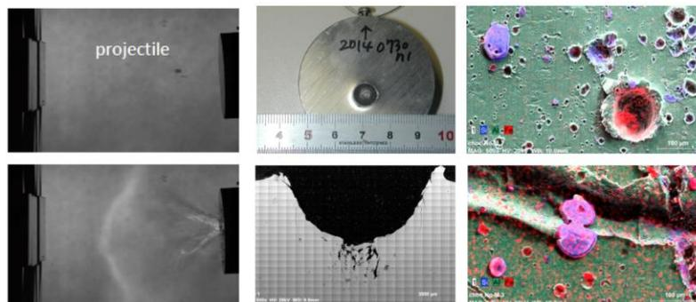
**Figure 3:** High velocity impact experiments on a metallic target with millimeter-sized basalt projectiles (left) using a two stages light gas gun (coll. Prof. A. Nakamura at the University of Kobe, Japan). In collaboration with CEMEF, target (center) and ejecta (left) are analyzed *post-mortem* for their microstructure and chemical composition. The ejecta (right), collected in an aluminium catcher were analysed for minor and trace elements using EDX-SEM and LA-ICPMS techniques.
