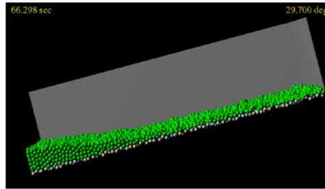
**Figure 2:** End-state of a simulation of a tilting bed with loose particles (green) on top of fixed particles (gray). Sustained flow initiates at a tilt angle of approximately 24 degrees for this configuration that used about 14,000 monodisperse 5 cm radius particles (half free, half fixed) on a 6 by 9 m bed. For this simulation, the static and rolling friction parameters are set to 0.1 (low friction).
