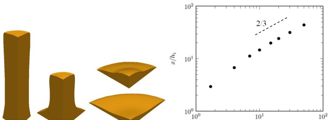
Figure 5:  $\mu(I)$  computation of the shape of a granular column at  $t = 20\%$ ,  $40\%$ ,  $60\%$  and  $80\%$  of total collapse and demonstration of the  $2/3$  scaling law of 2D relative spreading distance vs. initial aspect ratio.
