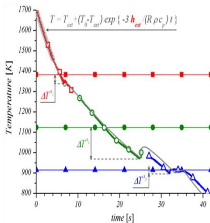
Figure 1. Cooling history of a levitated Ni-75at.%Al 6 mm diameter droplet (colored curve) measured and (grey) calculated (DLR, Köln, DE) [1].
