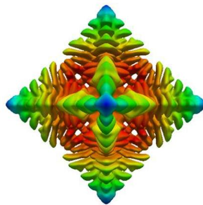
Figure 4. Phase field simulation of dendritic growth in an undercooled melt revealing the overall morphology of the primary solid phase formed from the melt [3].
