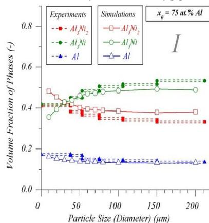
Figure 3. Fraction of phases (plain lines) predicted and (dashed lines) measured using neutron diffraction (Aix-Marseille University) in atomized particles [2].
