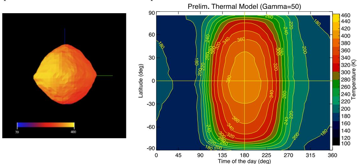
**Figure 4:** Left: Example of temperatures calculated on the radar shape model of the asteroid Benu. Right: Average surface temperatures calculated at 1 AU from the Sun assuming a value of the thermal inertia of  $50 \text{ J m}^{-2} \text{ s}^{-0.5} \text{ K}^{-1}$  using the Preliminary Thermal Model developed for the Mission Preliminary Design Review (PDR).
