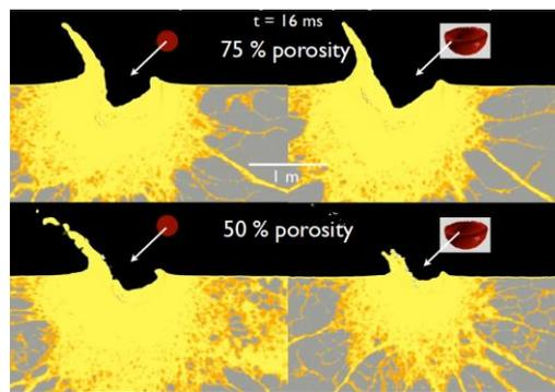
**Figure 3:** Snapshot of a SPH simulation of the hypervelocity impact performed by the SCI on the asteroid's surface as a function of porosity and projectile's shape (left : spherical projectile, right : shell). One can easily see the influence of those parameters on the crater's size/morphology and depth. The yellow zones correspond to damaged zones (from Michel et al. 2016).
