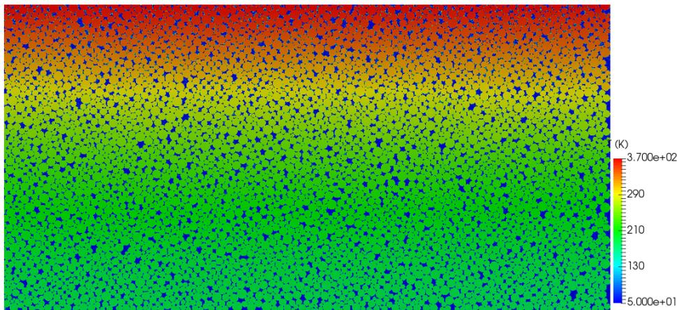
**Figure 5:** Temperatures in a very compact regolith bed calculated with a finite element thermophysical model that takes into account inter-grain conduction and the presence of voids.
