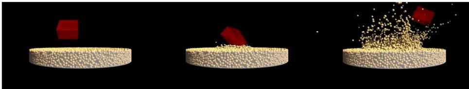
**Figure 2:** Snapshots from a simulation of MASCOT landing and bouncing on a surface composed of mono-size spherical particles (1 cm in diameter) in the gravity conditions of the asteroid Ryugu. In this run, the lander rotates on itself (1 rotation/mn) and impacts on an edge, before bouncing. Such a simulation allows measuring the coefficient of restitution as a function of the impact geometry and assumed surface properties. Here, MASCOT is modeled as a box with its actual moment of inertia.
