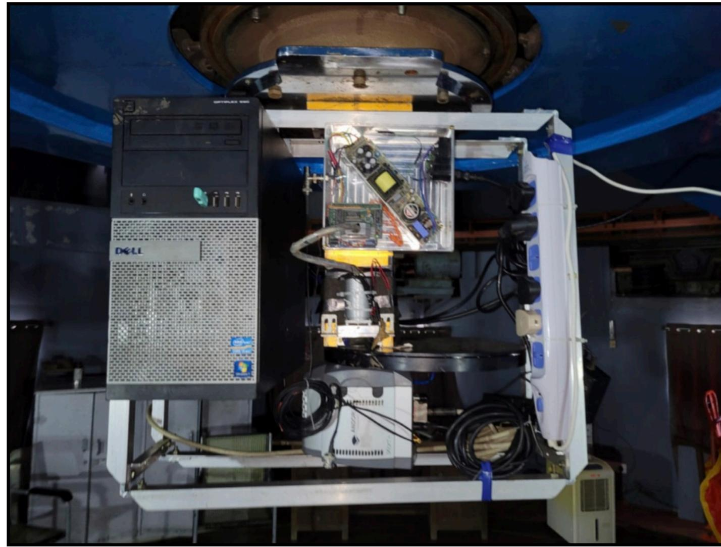
EMCCD based Polarimeter (EMPOL)
