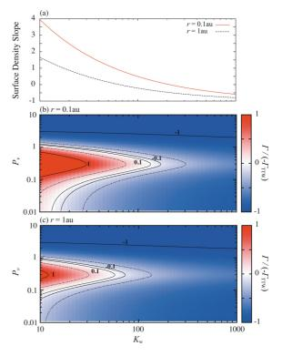
**Fig. 2.** Surface density slope in a steady state at r=0.1 au and 1 au for various values of  $K_{\rm w}$  (panel **a**)). Migration efficiency  $(\Gamma/(-\Gamma_{\rm TTW}))$  for planets with e=0.01 at r=0.1 au (panel **b**)) and r=1 au (panel **c**)). The contours show a migration efficiency of -1, -0.3, -0.1, 0.1, 0.3, and 1. When  $\Gamma > 0$ , planets move outward.
