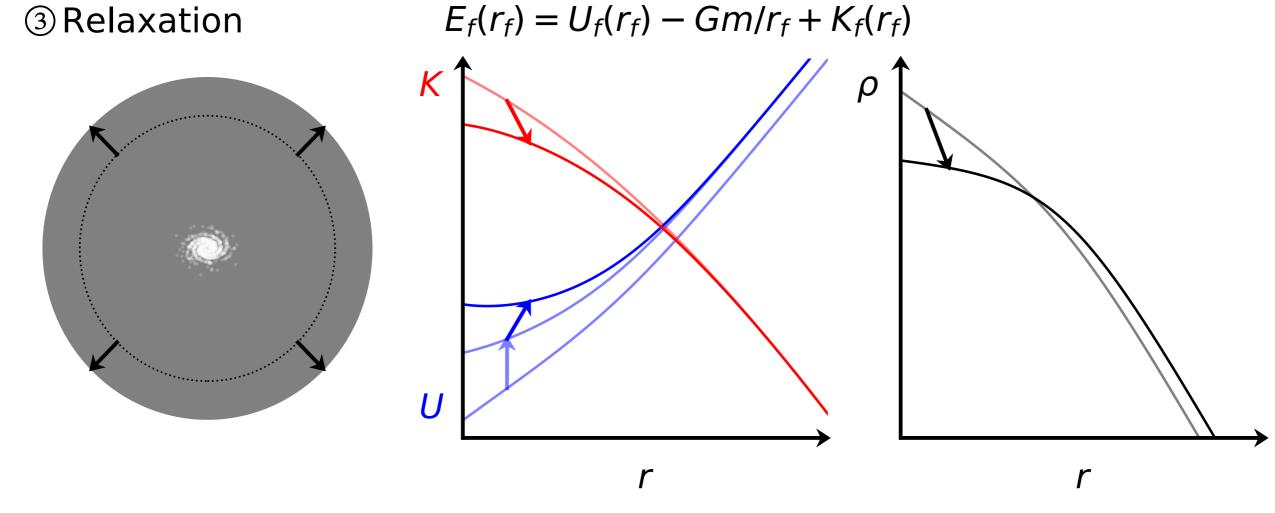
Given functional forms U(r;p,m) and K(r;p,m), energy conservation  $E_f(r_f) = E_i(r_i)$  during relaxation yields the final state
