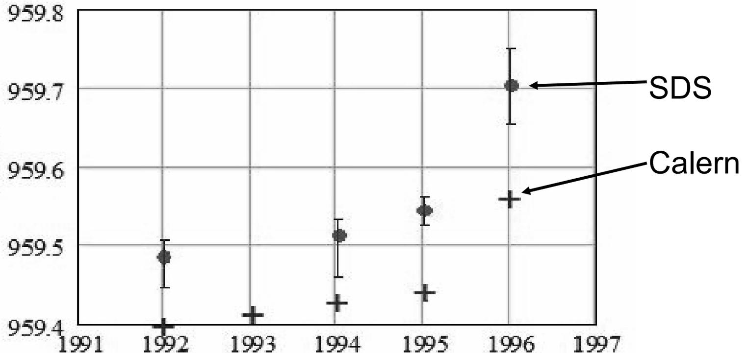
Results of four stratospheric balloons flights carrying SDS (Egidi et al., 2006) showing a diameter increase of 0.2" while the solar activity decreases.
