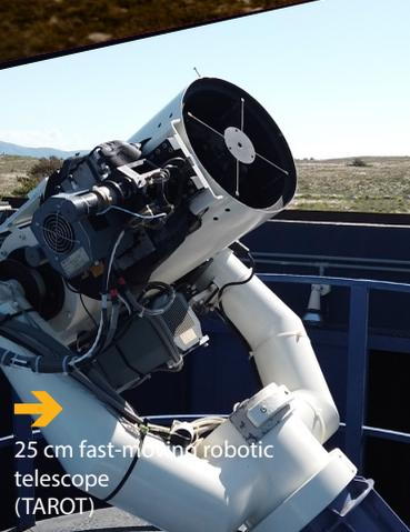
→ 25 cm fast-moving robotic telescope (TAROT)
